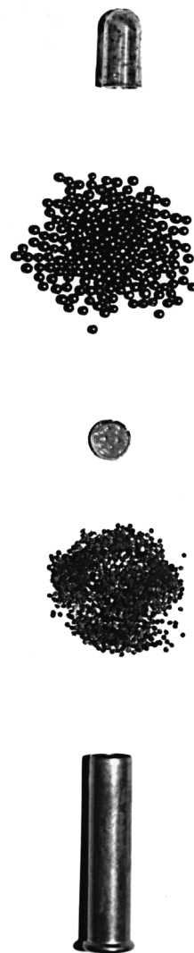
FIG. 2b—Disassembled shotshell cartridge showing from top to bottom; plastic cylinder, pellets, wadding, gunpowder, and cartridge casing.
