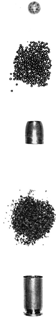
FIG. 1b—Disassembled Glaser safety cartridge showing from top to bottom; plastic plug, pellets removed from interior of copper jacket, copper jacket, gunpowder and cartridge casing.
